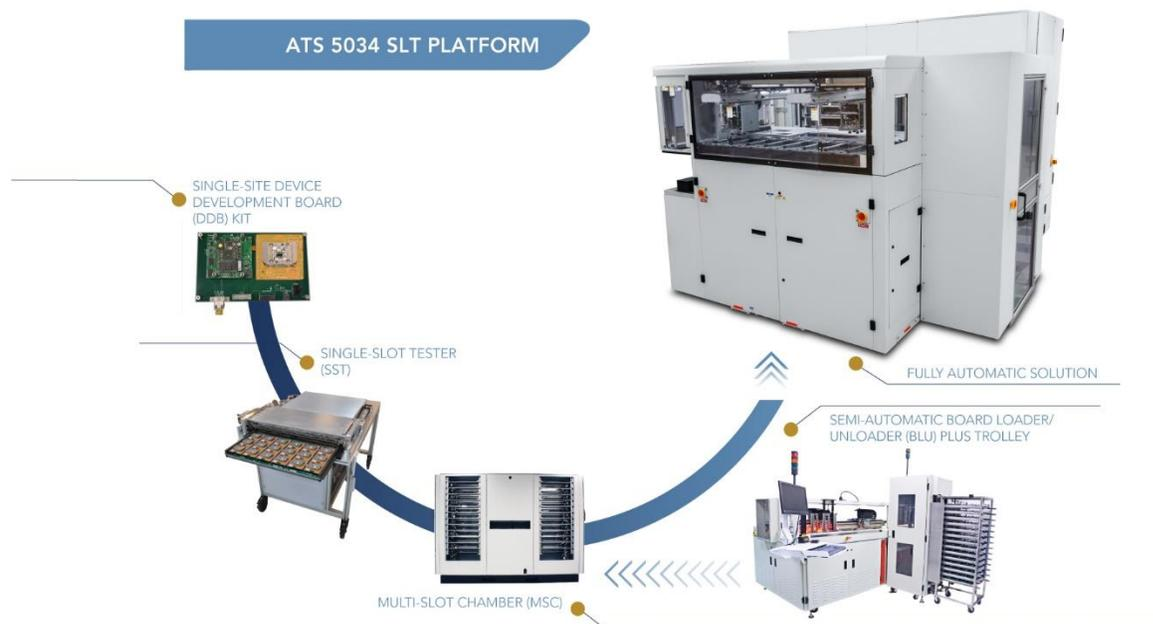
Detail view of the scalable options within the ATS 5034 SLT Platform system.
