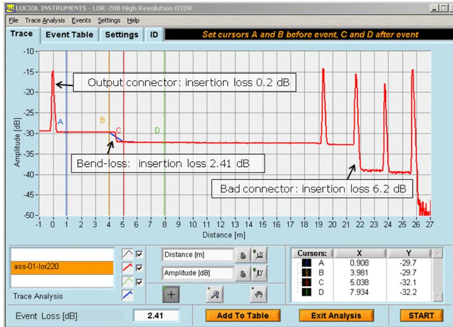
**Figure 2: A Typical trace obtained with the LOR-220**
